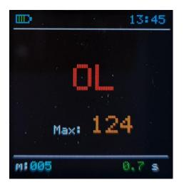
This message means that the measured value is higher than 125 standard scale division [Nrm].
