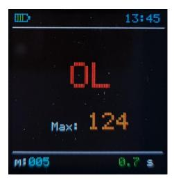
This message means that the measured value is higher than 125 standard scale division [Nrm].
